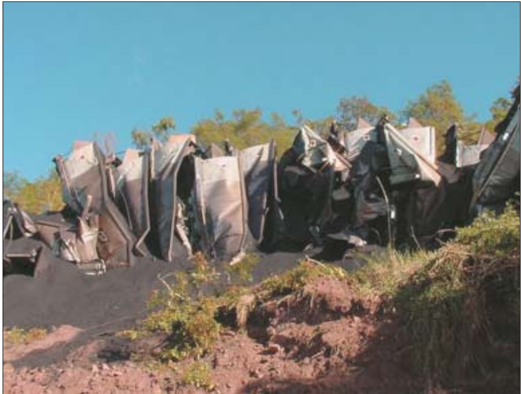
Figure 6: View of derailment site showing several wagons 'stacked' vertically
