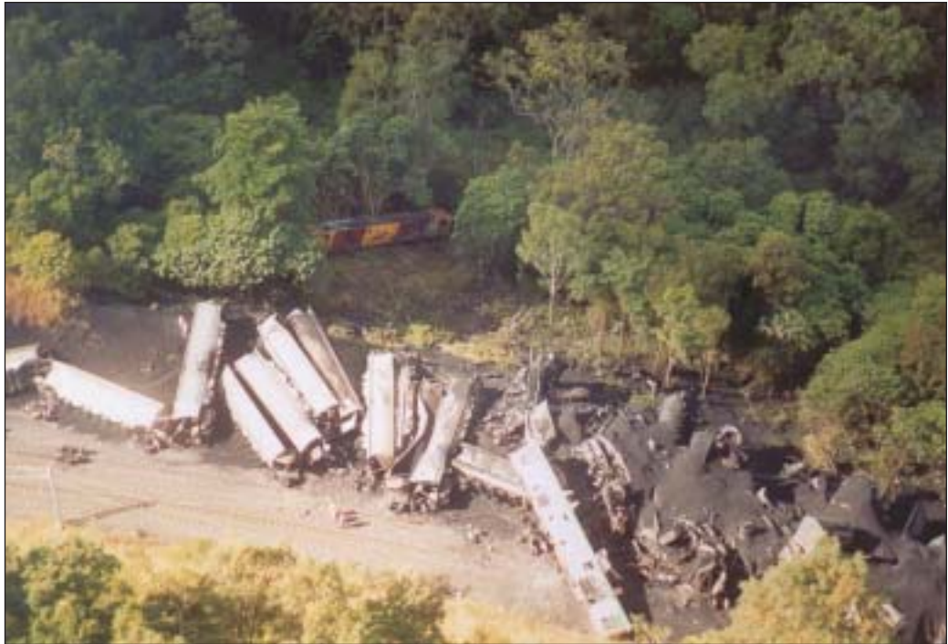
Figure 7: View of derailment site showing several wagons 'buried' under coal and other wagons
