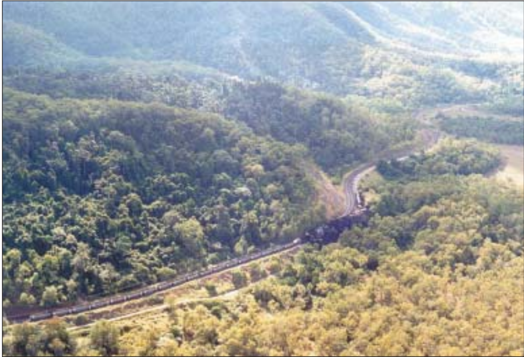
Figure 9: View of derailment site showing trailing 18 wagons, which remained on the track
