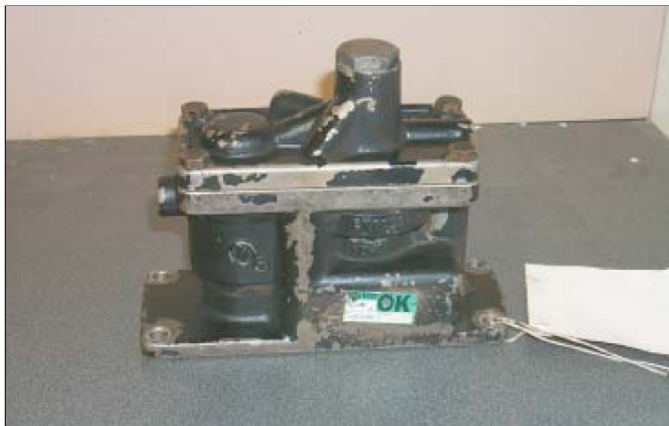
Figure 20: Brake Pipe Control Valve from ELRC119
